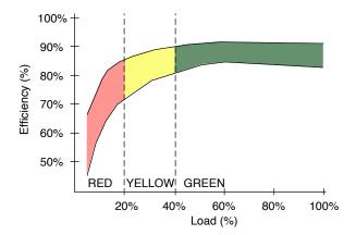
Figure 7: Power Supply Efficiency.
