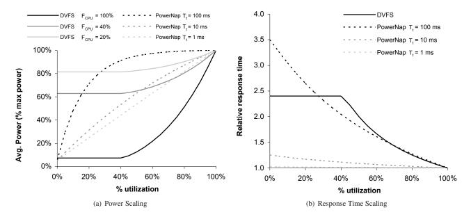
Figure 6: PowerNap and DVFS Power and Response Time Scaling.
