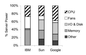
Figure 2: Server Power Breakdown. No single component dominates total system power.
