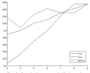
Figure 5. Comparison between correct classification rates for PCA/LDA+NN and the proposed *RBPCA MaxLike* classifier in ORL
