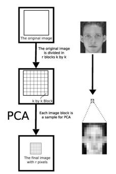
Figure 1. Illustrative diagram of the proposed Block-Based PCA.
