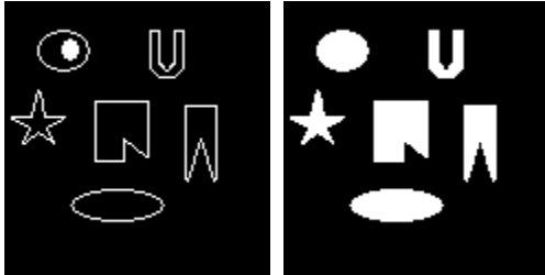
Figure 2. Example of the algorithm's operation for a binary image. The original image (to the left) is filled by the algorithm and the result can be seen in the resulting image to the right (auxiliary image).
