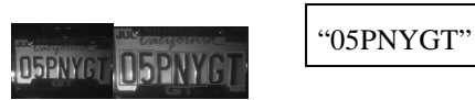
Figure 3. (a) One of the test video frames which have been used in the experiment, (b) results of the character segmentation technique, (c) the output of the OCR system.
