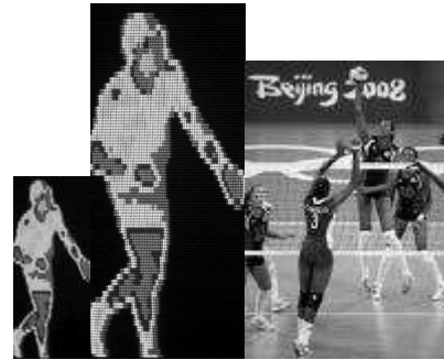
Figure 4. From left to right: the 160x120 thermal frame, super-resolved thermal frame, CCD camera frame.
