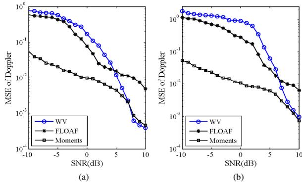
Figure 2. MSE of Doppler estimation in conventional and proposed methods (a) constant noise variance. (b) variable noise variance.
