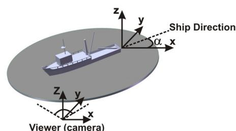
Figure 1. Angular direction of the ship in relation to the viewer coordinate system (referential).
