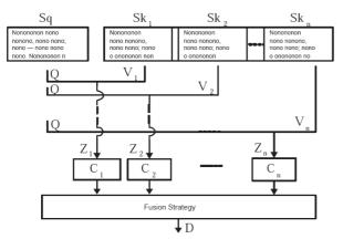
Figure 1. Architectur of the writer-independent model
