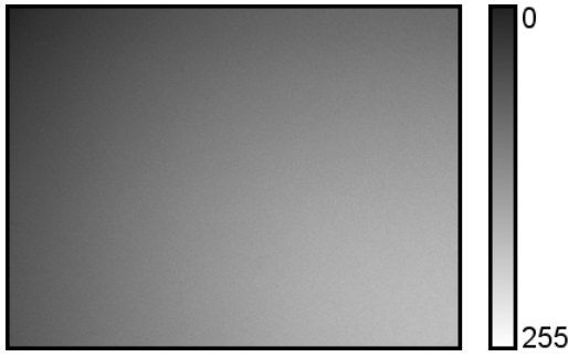
Figure 1. Upper left quarter of the red channel of the captured image when the monitor displayed only white pixels.
