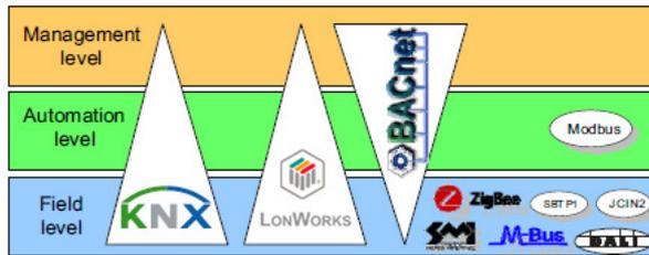
Figure 1. Standards in building automation [3]
