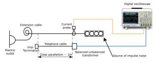
Figure 1. Setup of a workplace for impulse noise diagnostics.
