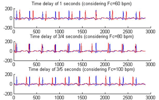
Figure 3. Original and delayed ECG with 1s, 3/4s and 3/5s of time-delays.
