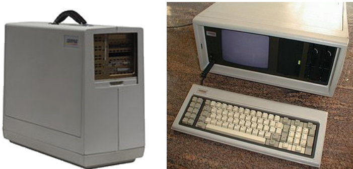
Figura 3.3 Compaq portable 1982, clone do IBM Personal Computer.
