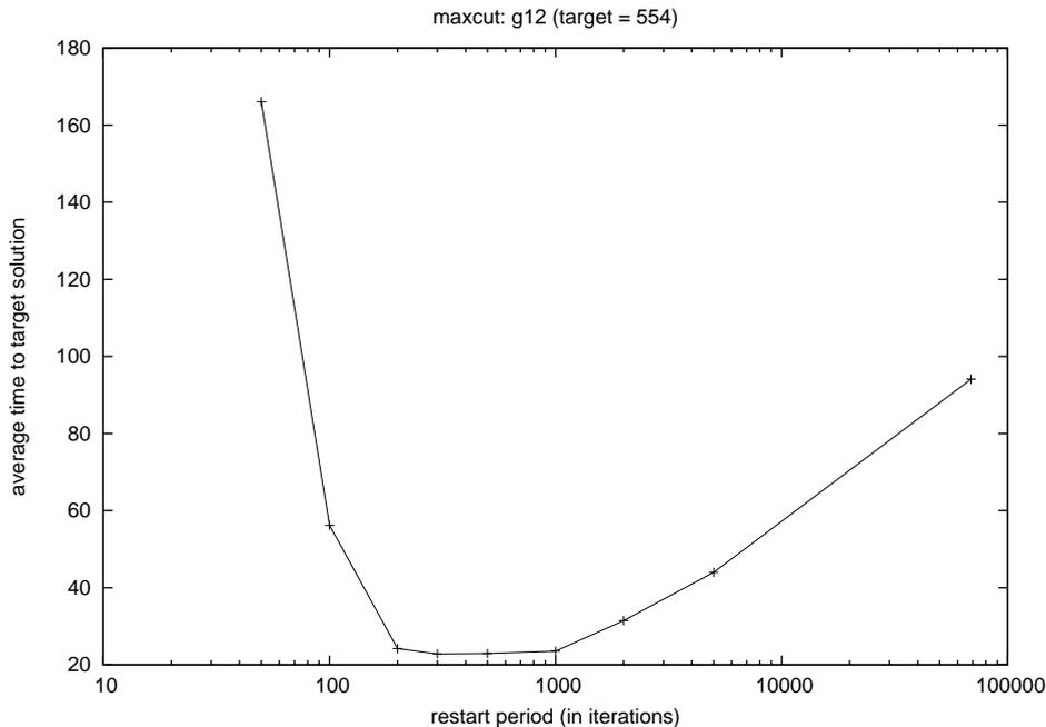
**Fig. 3.** Average time to find a cut of weight at least 554 for max-cut instance *G12* as a function of the restart parameter  $\kappa$ . The figure shows that the best values are in the range from 200 to 1000 iterations.
