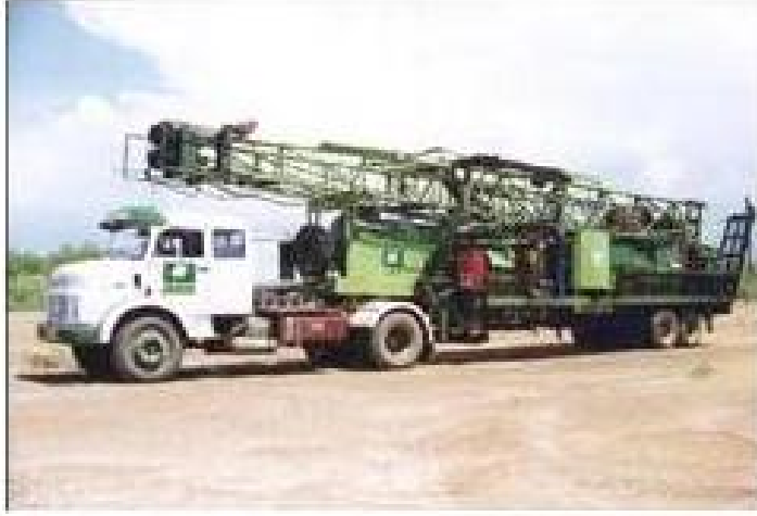
Fig. 2. Transportation of a workover rig
