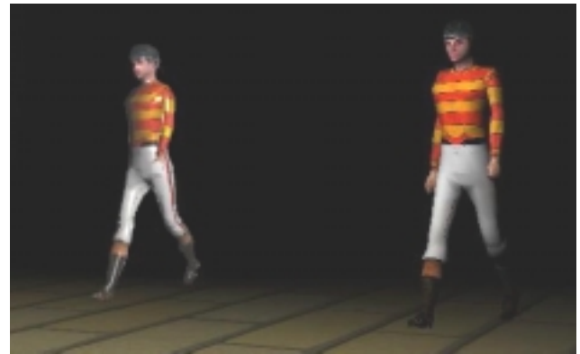
Figure 6. The character at the left side is being rendered by the software shader and the character at the right is entirely rendered by GPU.
